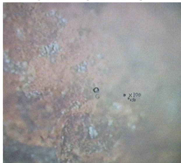
Figure 2: Typical optical image of fresh broken surface of the Sharyn-Gol coal sample
