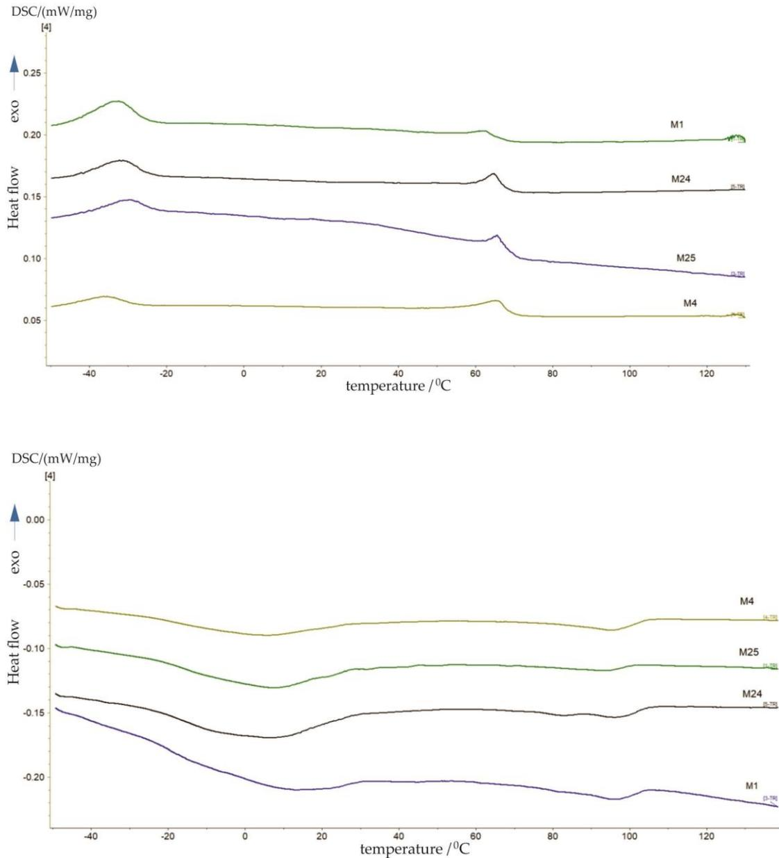
Fig. 4. Calorimetric curves obtained during cooling (a) and heating (b) of porous Ni-Ti samples obtained by SHS without ultrasonic activation (M1) and 5  $\mu\text{m}$  (M24), 15  $\mu\text{m}$  (M25) and 25  $\mu\text{m}$  (M4)
