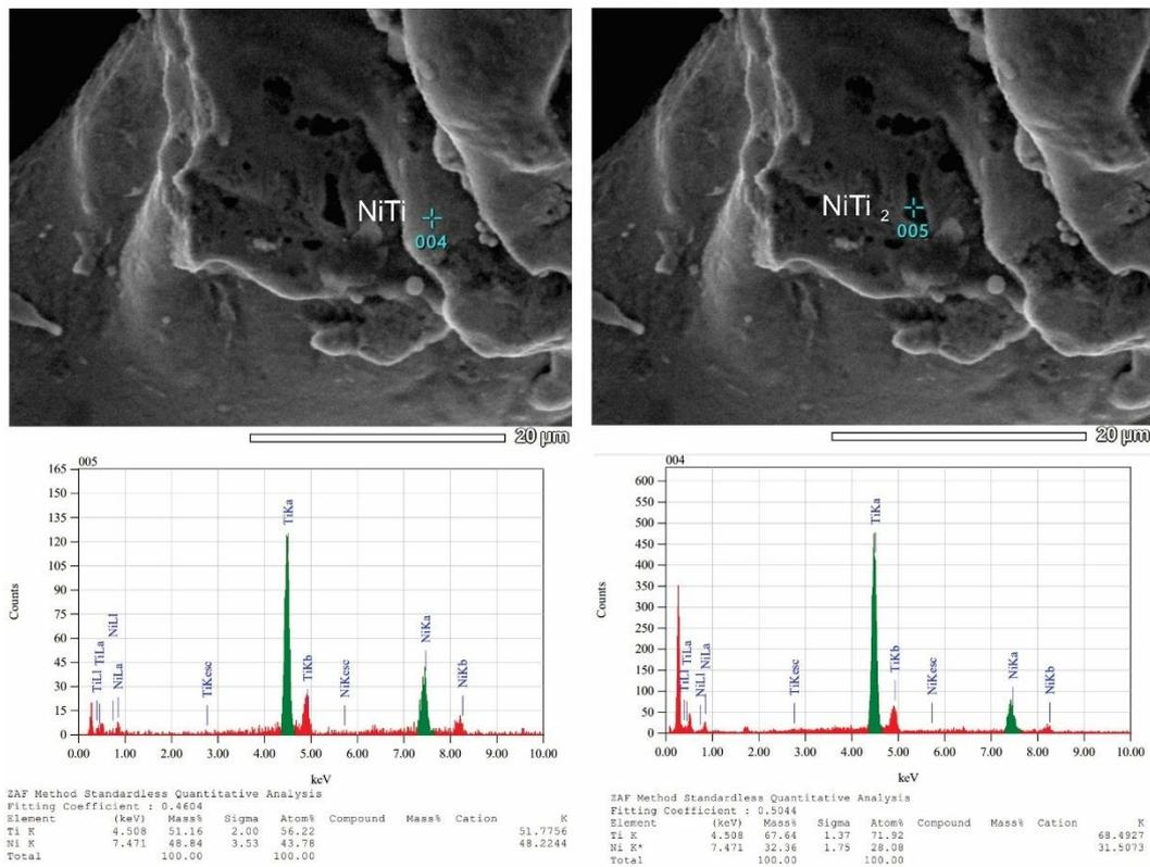
Fig. 2. Microstructure and EDS results of sample ultrasound treated for amplitude of 5  $\mu\text{m}$
