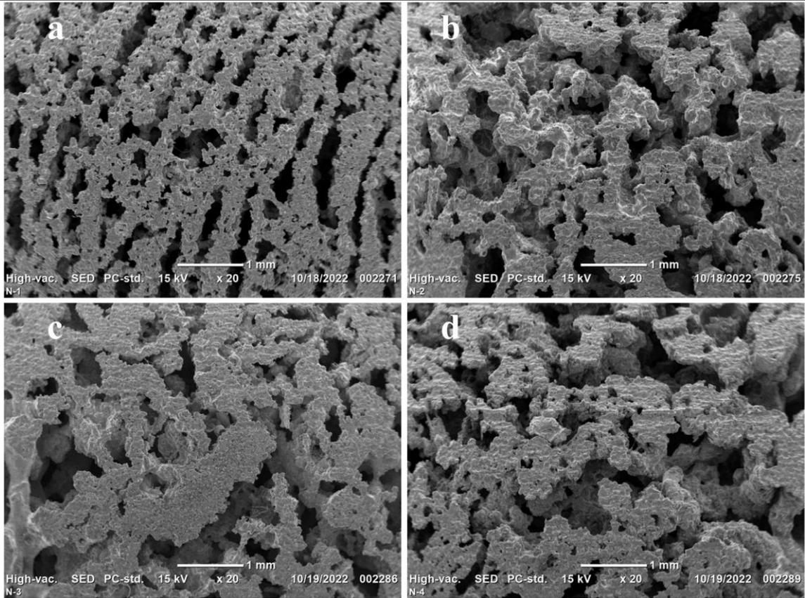
Fig. 1, Microstructure of porous Ni-Ti alloys ultrasonic activation for amplitude: (a) Not treated by ultrasonic, (b) 5  $\mu\text{m}$ , (c) 15  $\mu\text{m}$ , (d) 25  $\mu\text{m}$
