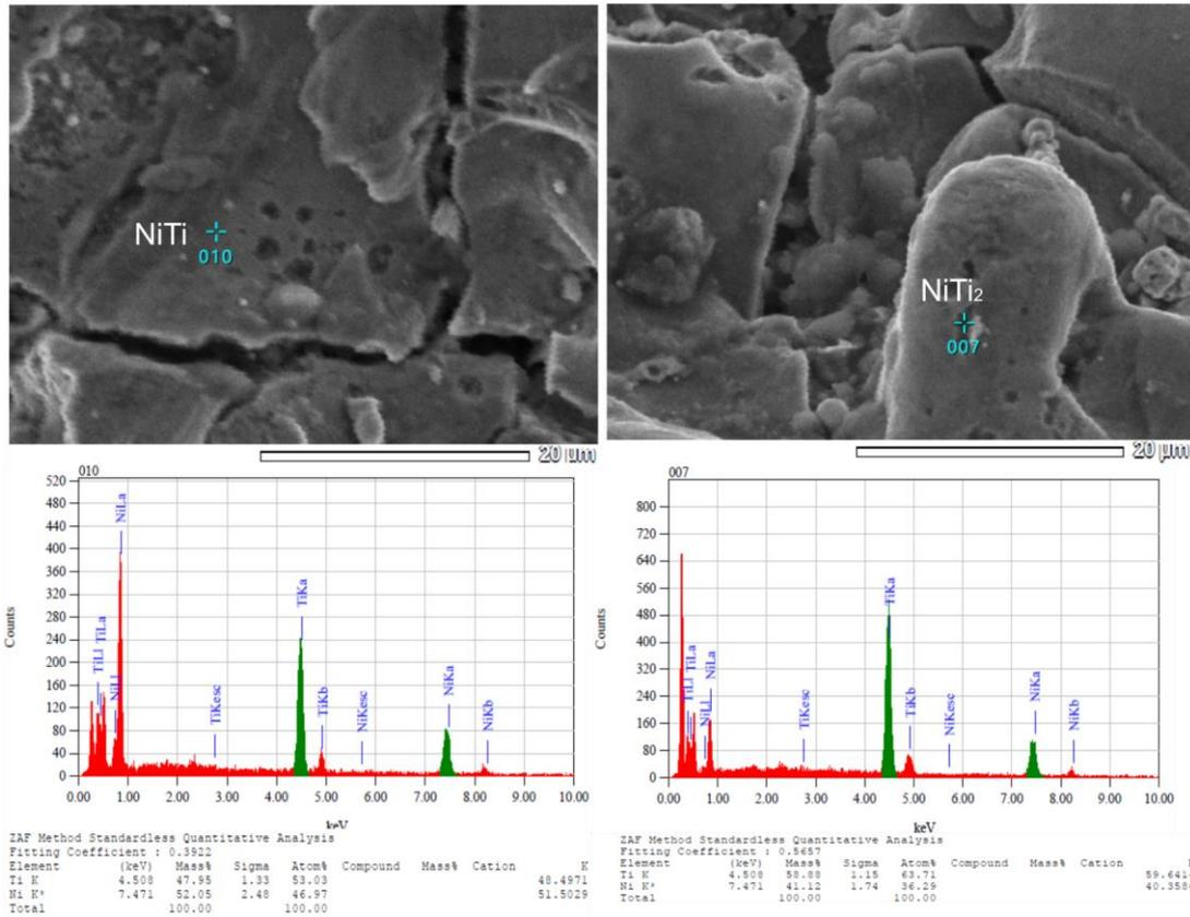
Fig. 3. Microstructure and EDS results of sample ultrasound treated for amplitude of 15  $\mu\text{m}$
