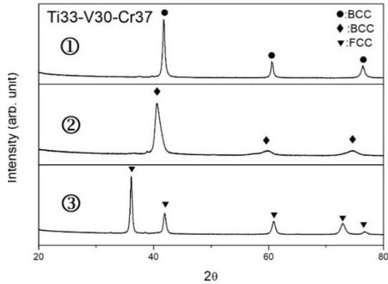
Fig 6. XRD pattern for three main points.
