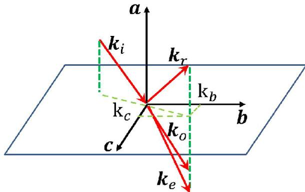
Figure 1: Double refraction at boundary of an  $a$ -cut uniaxially crystal surface
