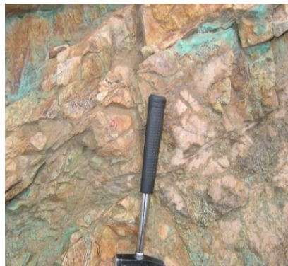
Photo.9. Rhyolite with malachite coatings at cracks veinlets and inclusions
