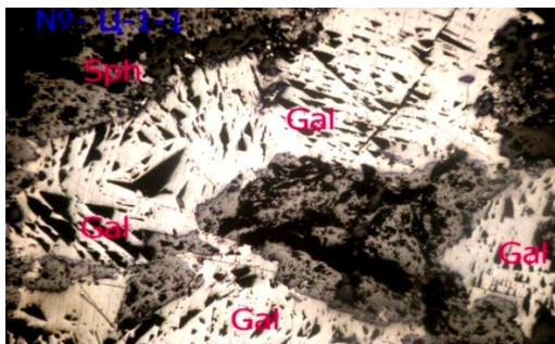
Fig. 2. Polished block Borehole ID 1-1. Irregular, long extended grains of galena (white) within Sph- sphalerite (whitish grey); Gal- black triangle is clearly visible within galena Magnification 5x.
