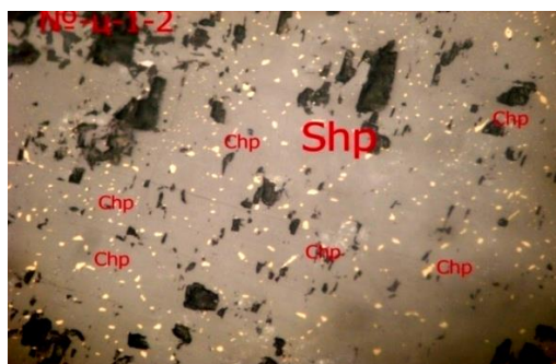
Fig. 3. Polished block Borehole ID -1-2 small emulsion-like grains of chalcopyrite (greenish pale) in sphalerite (whitish grey) magnification 200x.
